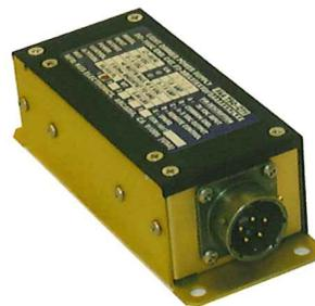
KGS Electronics light dimming power converters utilize a pulse width-modulated (PWM) DC to DC power conversion topology to provide controlled and regulated DC output power. These converters transform unregulated 28 VDC input to variable and regulated output power. The output voltage is adjusted via an external remote control rheostat, potentiometer or externally controlled voltage reference. All DC power converters provide full regulated output voltage, overload protection and current limiting.
